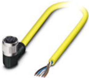
Sensor/Actuator cable, 5-position, PVC, Yellow RAL 1021, Free cable end, on Socket angled M12-SPEEDCON, A-coded, Cable length: 10 m
